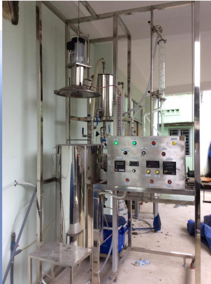
Herb extraction and steam distillation system
